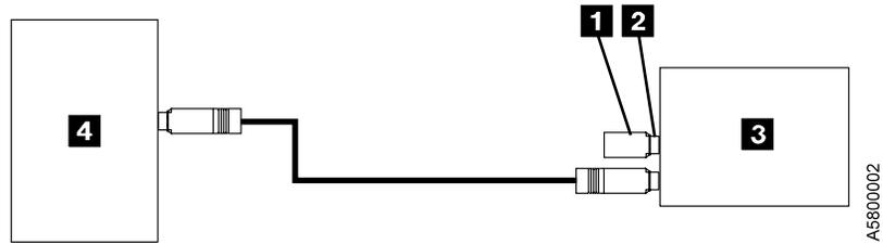
Figure 6. Attaching a Terminator to the 7208 Tape Drive. The view is from the side. The thumbscrews are not shown.
